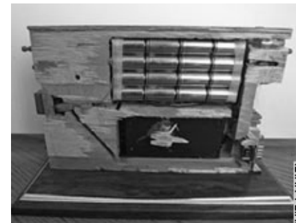
This is part of a British MI5/PSNI bugging device found hidden in the floorboards of a Sinn Fein office in Belfast in September 2004. Approx 10.5 inches by 6.5 inches.
